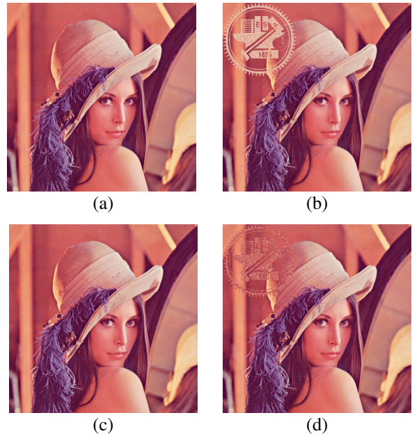
Figure 3 An example of results of applying proposed method. (a) A color image of "Lena". (b) Stego-image after embedding visible watermark of size 200×200. (c) Losslessly recovered image from (b). (d) Lossy recovered image without a right key.
